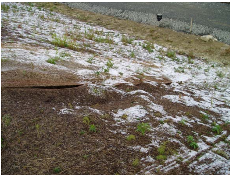
Figur 35. Erosion under halmmattan i yta B.
