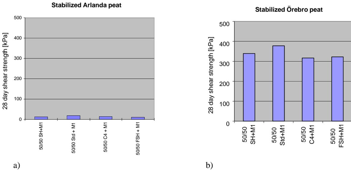
**Fig. 15. Shear strength after storage for 28 days. 250 kg stabilizer per m<sup>3</sup> was used unless otherwise indicated. Results normally represent the average of two specimens.**
