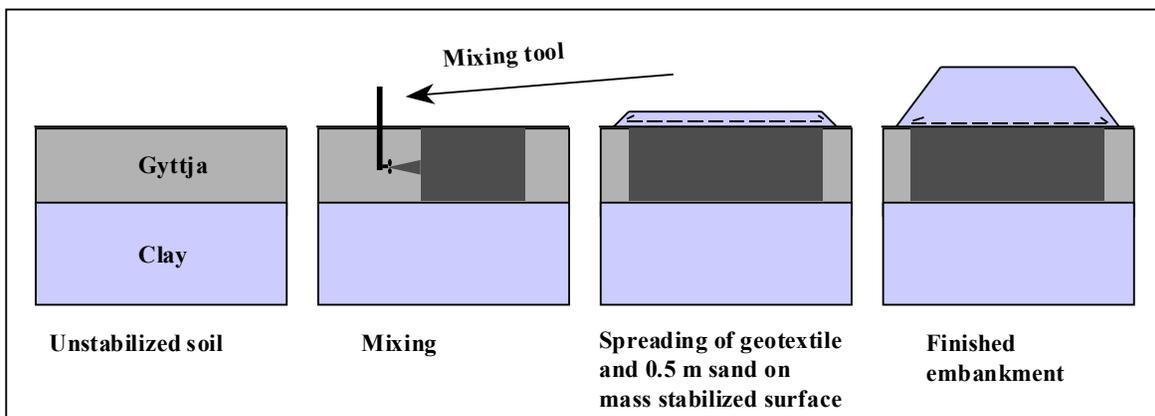
**Fig. 1. Mass stabilization.**
