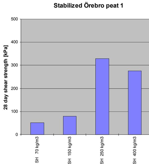
**Fig. 17. Shear strength after storage for 28 days. Tests using 250 kg stabilizer per m<sup>3</sup> were done on two parallel specimens, the results above representing the average. Other tests were done on single specimens.**
