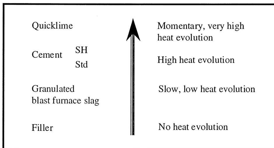
Fig. 4. Heat development in soil after stabilization with variout stabilizers.
