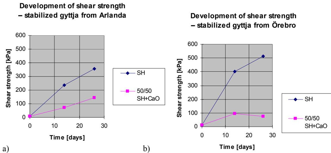
**Fig. 6. Strength evolution on stabilization with rapid hardening cement alone and with rapid hardening cement and lime. 200 kg stabilizer per m<sup>3</sup> was used in all specimens.**
