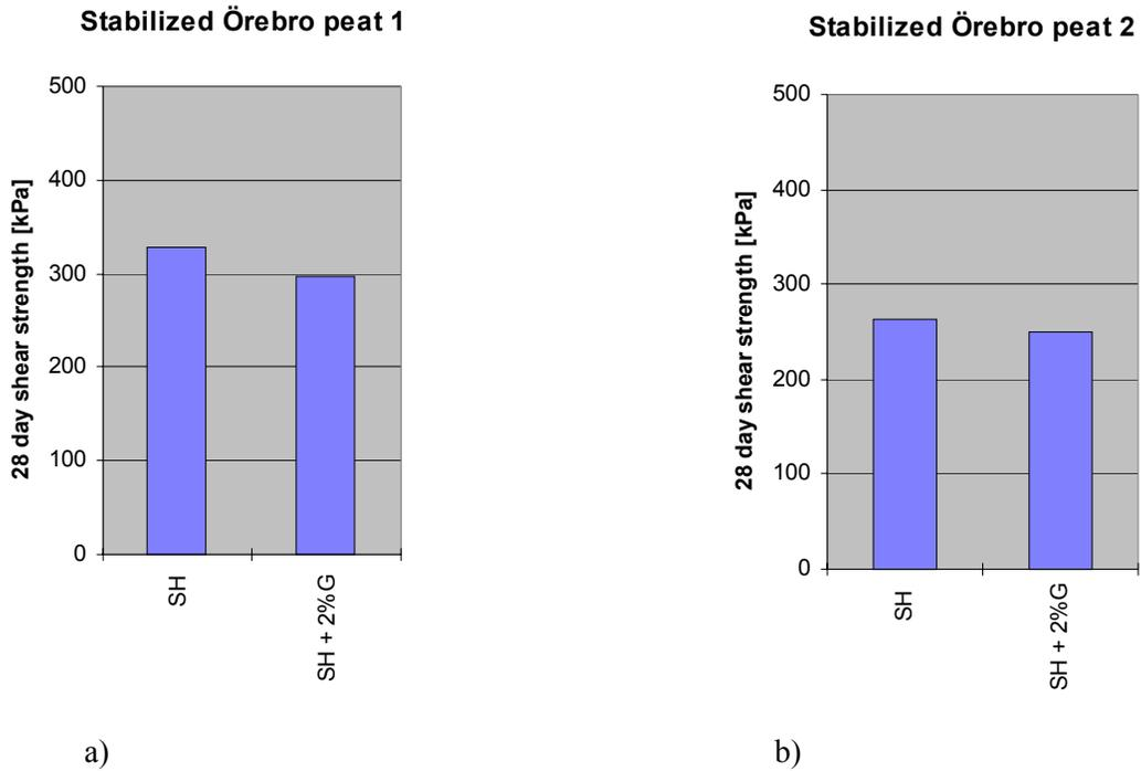
**Figur 16. Effect of Glorit on stabilization effectiveness in peat. 250 kg stabilizer per m<sup>3</sup> was used. Results normally represent the average of two specimens.**
