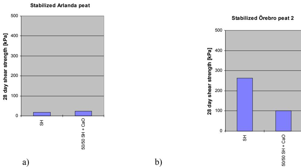
**Fig. 12. Shear strength on stabilization with jet cement alone and with rapid hardening cement and lime. 250 kg stabilizer per m<sup>3</sup> was used unless otherwise indicated. Results normally represent the average of two specimens**
