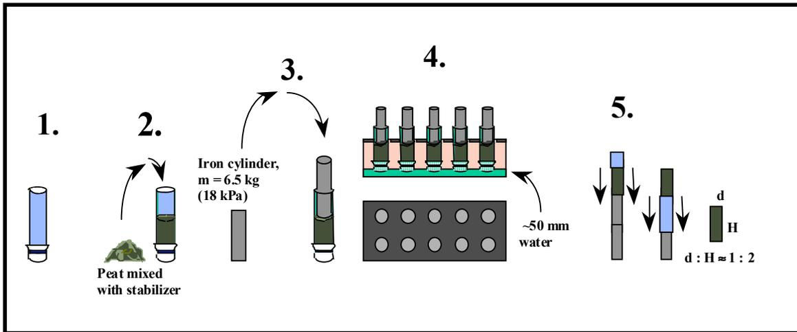
**Figure 3. Mixing and storage procedure in peat tests.**
