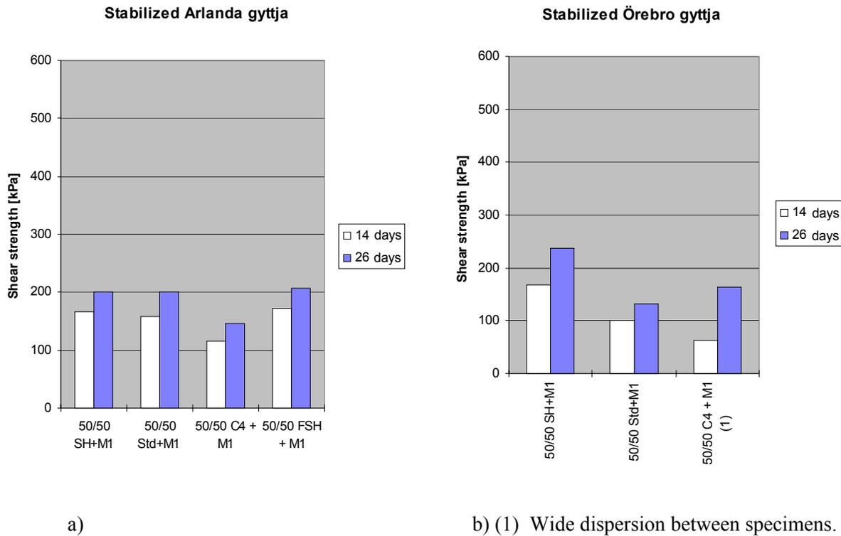
**Fig. 8. Shear strength of gyttja after storage for 14 and 26 days. The 26 day results are averages of two specimens. 200 kg stabilizer per m<sup>3</sup> was used in all specimens**
