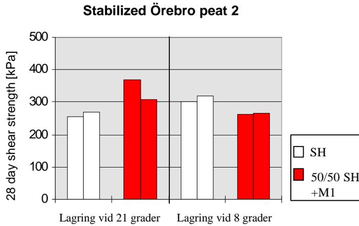
**Fig. 14. Comparison of stabilized Örebro peat stored at 8 °C and at 21 °C. 250 kg stabilizer per m<sup>3</sup> was used unless otherwise indicated.**
