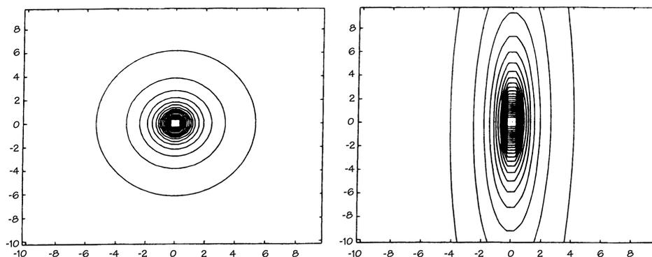
**Fig. 3.** Iso-displacement lines for the surrounding soil when the force moves from left to right in the figure with 25 % of the Rayleigh wave velocity (left) and 98 % of the Rayleigh wave velocity (right).
