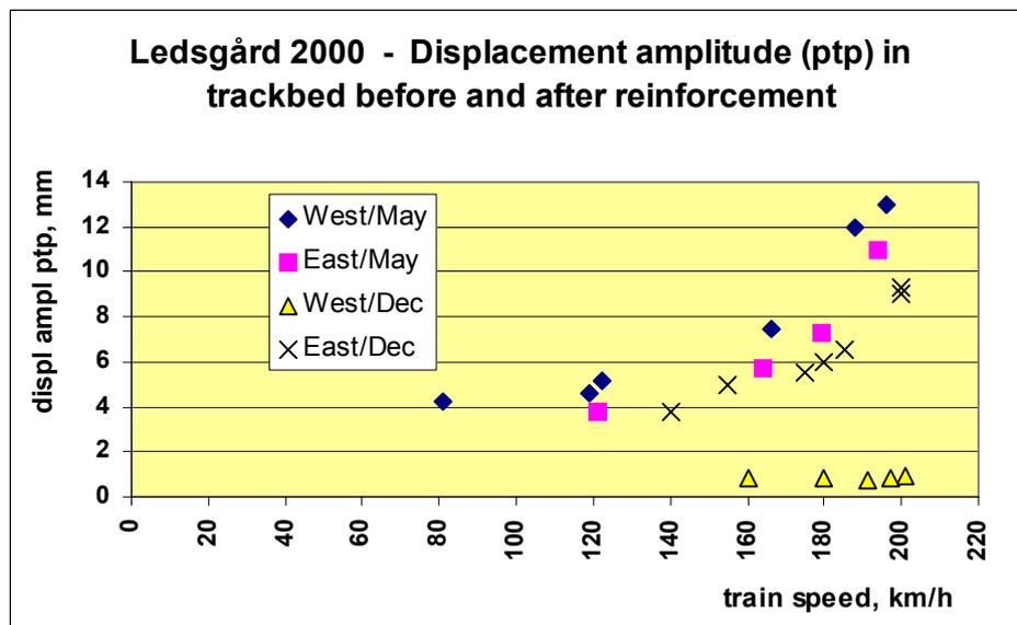
Fig. 23. Summary of measured displacements in the trackbed before (May) and after (December) reinforcement of the western track. Central part of X2 trains, J&W (2001).
