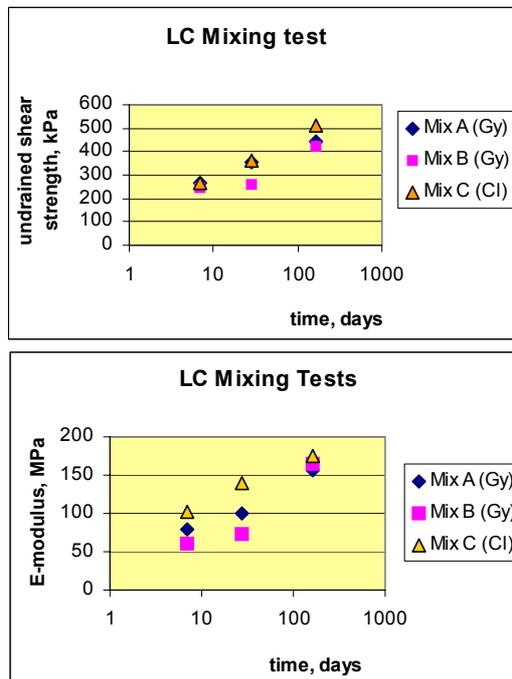
**Fig. 9.** Results of unconfined compression tests on lime/cement laboratory mixed samples of gyttja (Gy) and clay (Cl) ( $150 \text{ kg/m}^3$  lime/cement in a proportion of 25/75).
