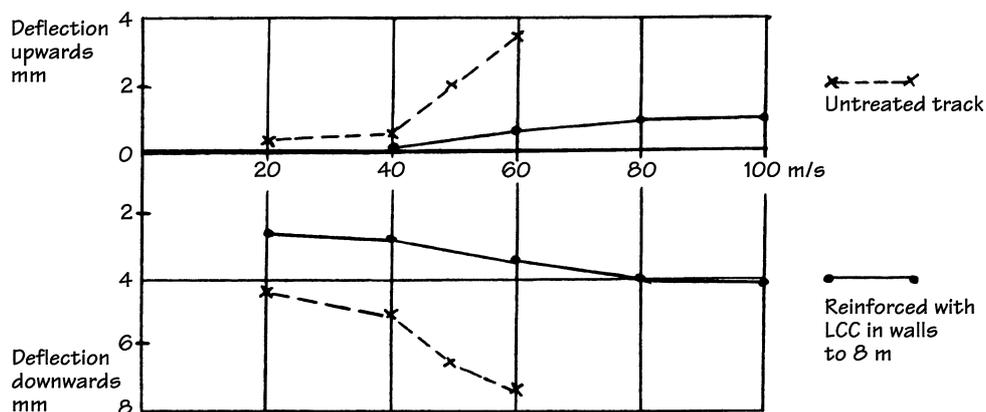
**Fig. 12. Summary of FLAC3D analyses at Ledsgård. Vertical displacement, upwards and downwards, under the moving load of two bogies. Untreated track and track stabilised by columns in walls (LCC = Lime Cement Columns).**
