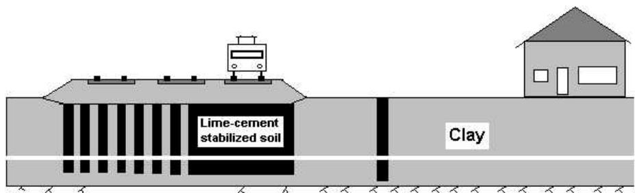
**Fig. 14. Principle of improvement of the soil beneath the track with the dry deep mixing method.**
