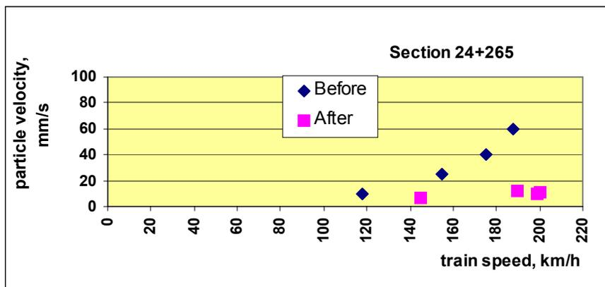
**Fig. 26. Particle velocity vs train speed in Sections 24+075, 24+175 and 24+265 before (May 2000) and after (December 2000) dry DMM improvement of the railway structure, J&W (2001).**
