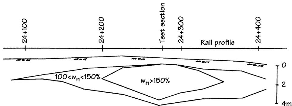
Fig. 6. Extent of the gyttja pocket along the track based on sampling at ten points. Natural water content indicated.
