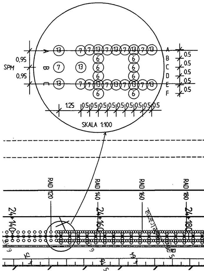
Fig. 13. Layout of soil improvement with the dry DMM columns (lime/cement columns). Also showing the transition at 24+150 from “settlement” stabilisation (from 24+100 to 24+150) and “high-speed” stabilisation. Column length below rail level given by figures within circles.
