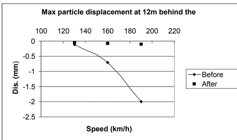
Fig. 29. Comparison of ground vibrations before and after installation of the dry DMM barrier with train speed, KTH (2001). Train traffic on the unreinforced western track.
