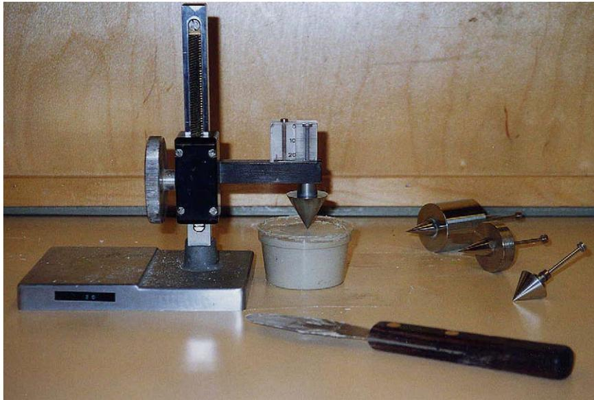
Figure 3.7 Fall-cone test apparatus.
