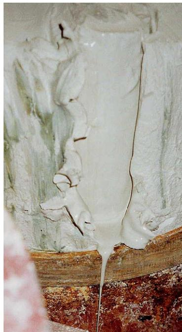
Figure 5.4 Example of a liquefied boundary layer. Column G, containing 7% lignosulphonate.
