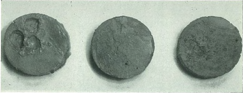
FIG. 2. Test specimens treated with (from left to right): humic water + 0.5 per cent NaOH; humic water; humic water + 0.5 per cent HCl.
