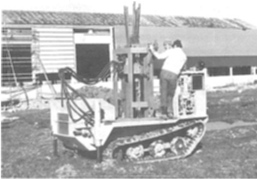
Fig. 1 Banddrivet fordon med plattform för borrhutrustning Tracked vehicle with working platform and boring equipment
