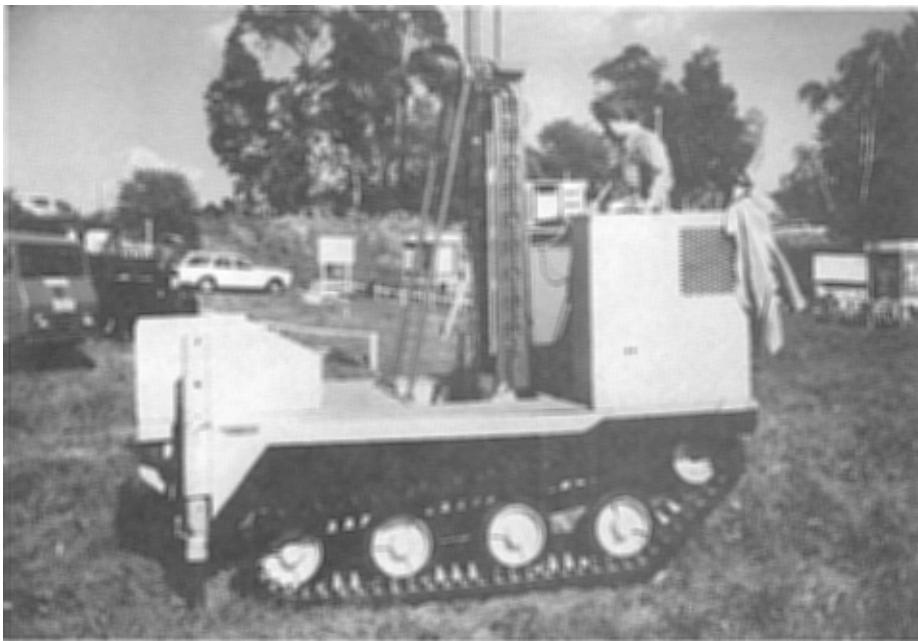
Fig. 3 Borrtrusning monterad på en bandvagn The boring equipment mounted on a tracked vehicle
