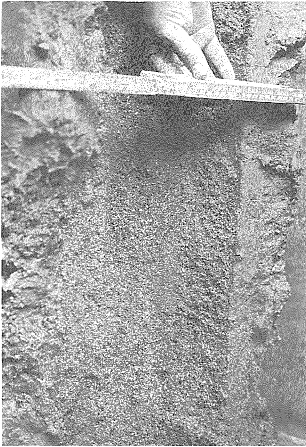
Fig. 7. Section of sand drain in the dry crust.
