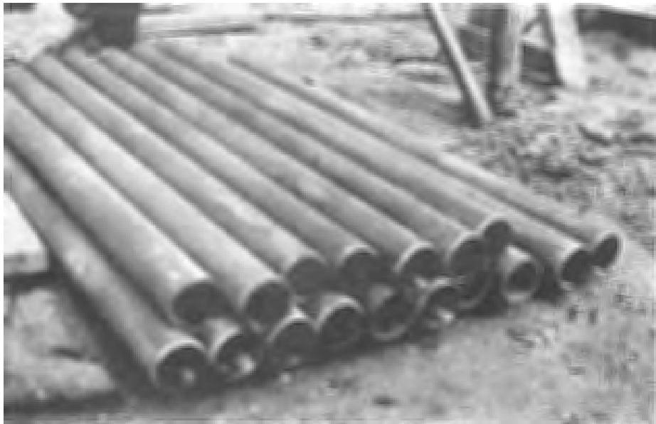
Fig. 3. The investigations were made on steel piles with 89 mm outside and 79 mm inside diameter. The pile segments before welding are shown above.
