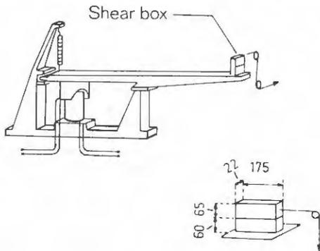
Fig. 6. Test Equipment for Determination of Soil Shear Strength With and Without Vibrations Used by Mogami & Kubo (1953).
