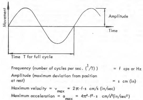
Fig. 3. Definition of Frequency, Amplitude, Velocity and Acceleration for a Sinusoidal Oscillation
