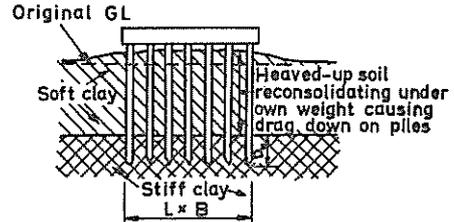
Fig. 2.4.1 Effects of ground heave on groups of driven piles in clay
