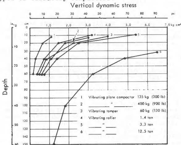
Fig. 8. Vertical Dynamic Stresses at Different Depth Under Vibratory Compactors of Different Types and Sizes According to Forssblad (1965)
