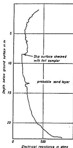
Fig. 10. Location of slip surface with the salt sounding tool.
