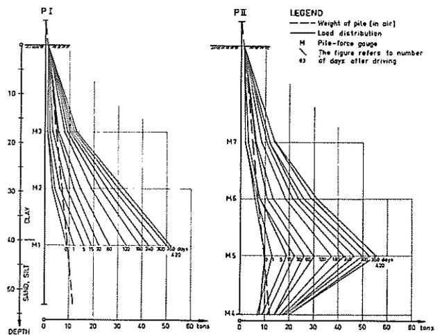
Fig. 2 Vertical distribution of load at different times after driving
