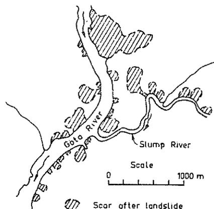
Fig. 2. Landslides at Utby.
