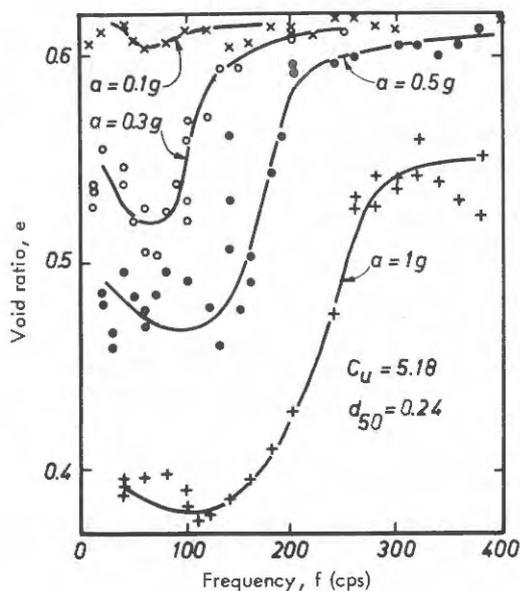
Fig. 10. Compaction of Dry Coarse Sand After Schäffner (1962)
