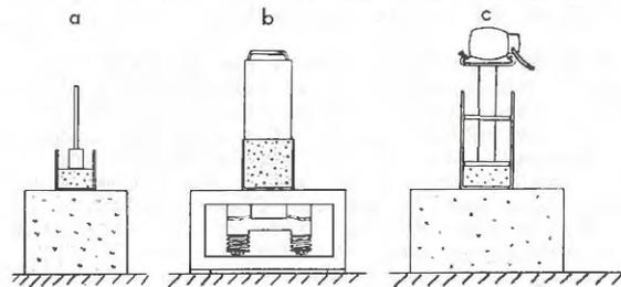
Fig. 1. Laboratory Compaction Methods a) Proctor Compaction Test; b) Vibratory Compaction Test with Vibrating Table and Surcharge Load; c) Vibratory Compaction Test with Vibrating Tamper or Hammer
