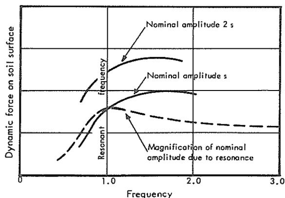
Fig. 5. Effect of Frequency and Amplitude on Vibratory Compaction of Soil
