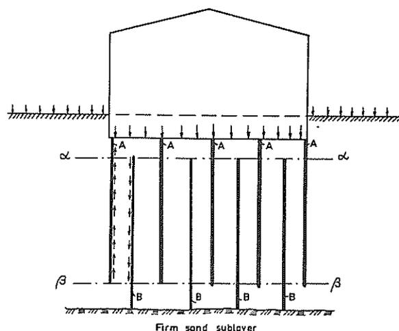
Fig. 2.2.1 Combination of friction and end bearing piles. A = friction pile. B = end bearing pile.
