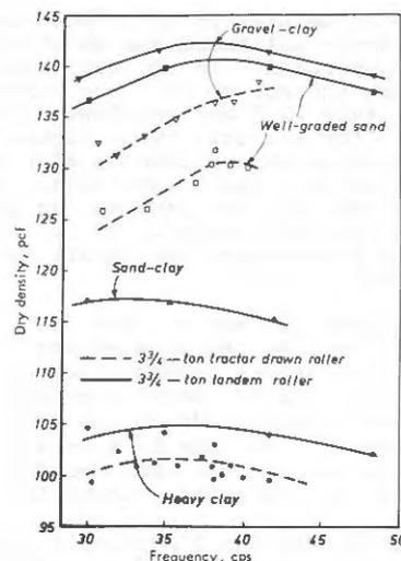
Fig. 9. Relationship Between Dry Density of the Compacted Soils and Frequency of Two Types of Vibrating Roller According to Lewis (1961)
