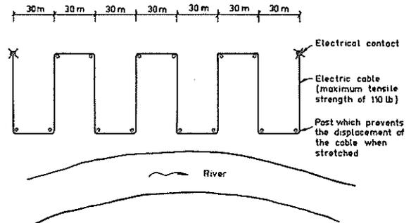
Fig. 16. Slide warning system type Swedish State Railways.
