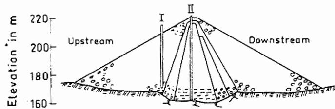
Fig. 1 Settlements in an earth and rockfill dam determined by means of nuclear measurements
