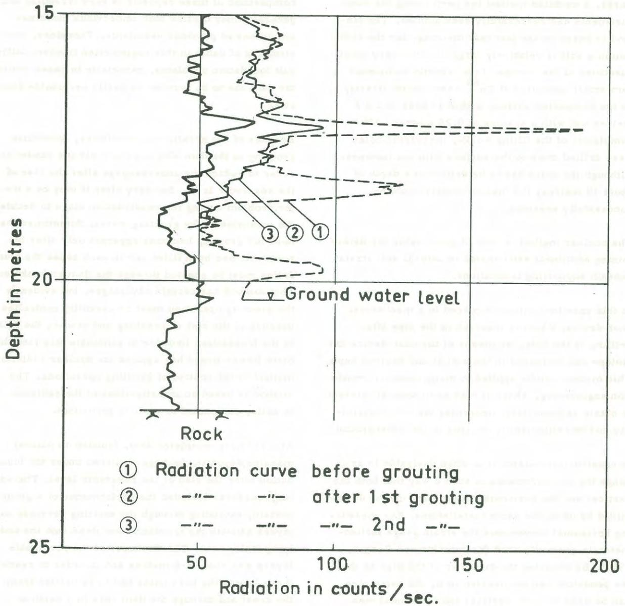
Fig. 2 Radiation curves, measured in foundation soils under a dam
