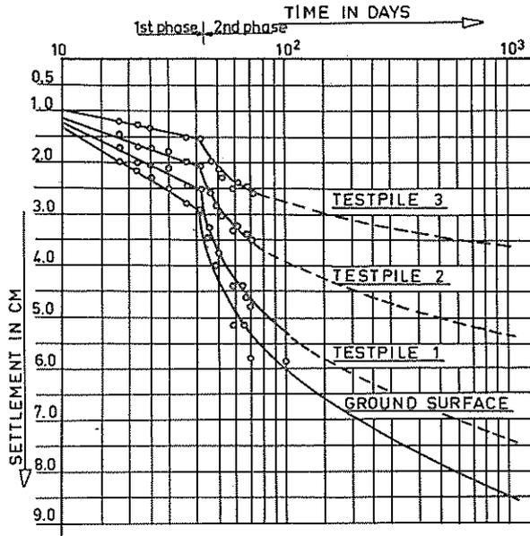
Fig. 2.3.1. Settlement-time relation for the ground surface and the 3 test piles during the two stages of the ground-water lowering. (After Weele, 1964).
