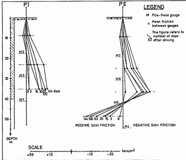
Fig. 8 Calculated average skin friction at different times after driving
