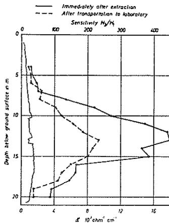
Fig. 4. Relationship between conductivity and sensitivity.
