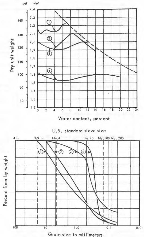
Fig. 2. Compaction Curves Obtained with the Modified AASHO Method and Grain Size Distributions for Different Types of Sandy Soils
