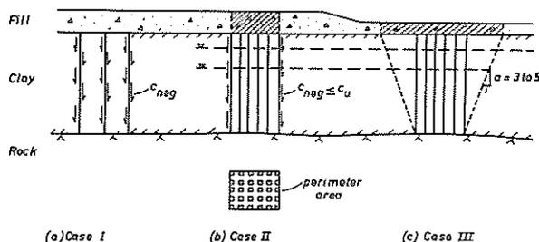
Fig. 1 Calculation of negative skin friction
