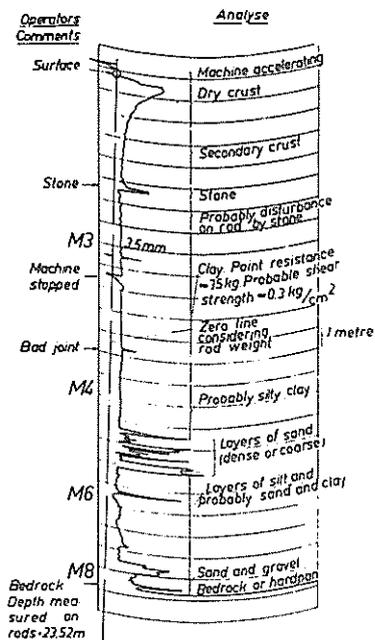
Fig. 7. Penetrometer record.
