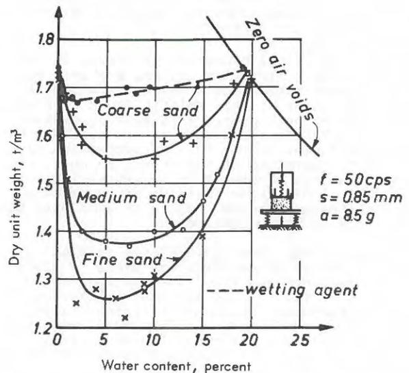
Fig. 7. Vibratory Compaction of Sand at Different Water Contents After Kutzner (1962)
