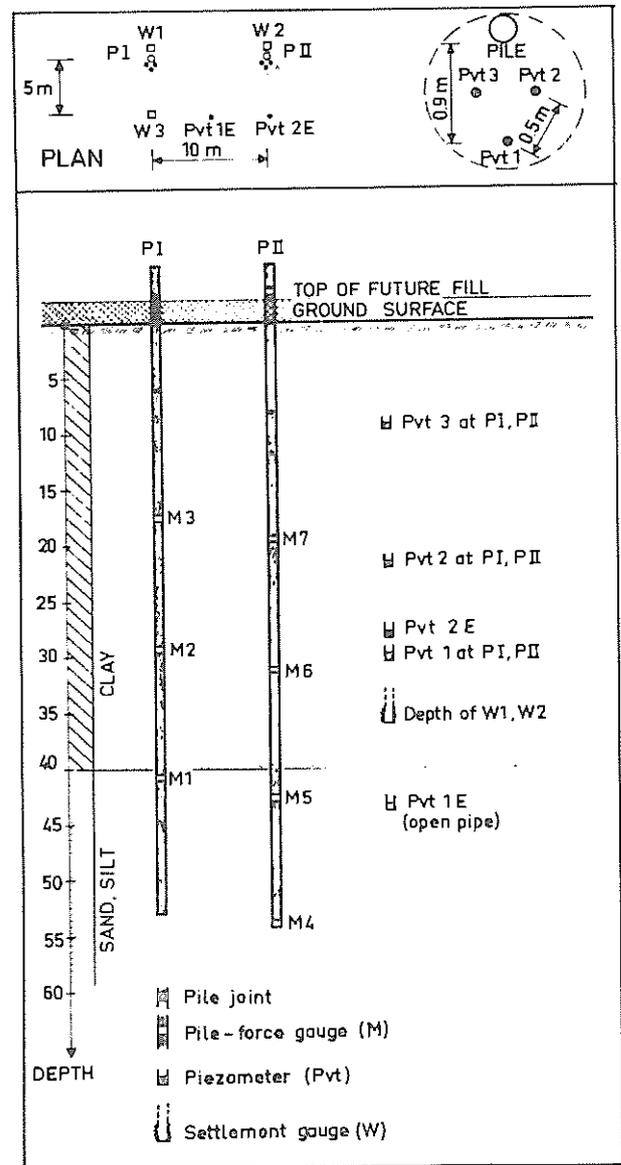
Fig. 3 Location of piles and instrumentation
