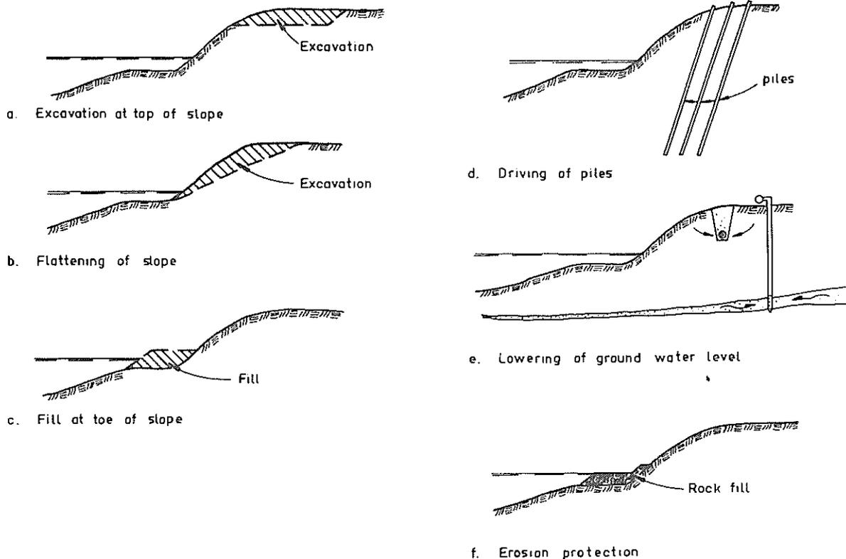
Fig. 12. Stabilization of slopes.
