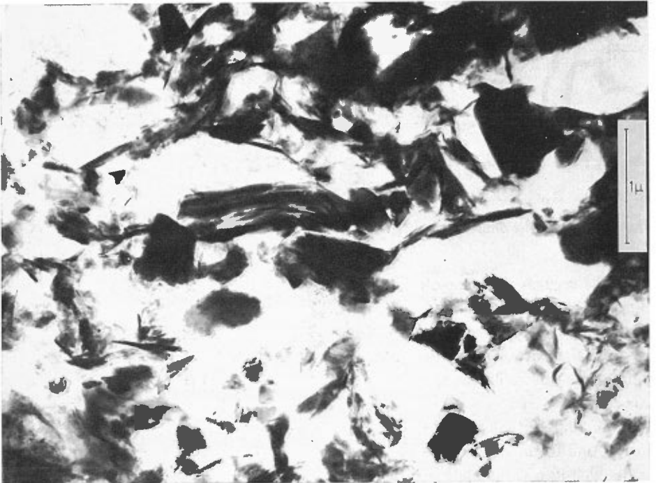
Fig.2. Vertical section through a quick clay (sample 4643 : 2). Electronic magnification \times 8,000 .
