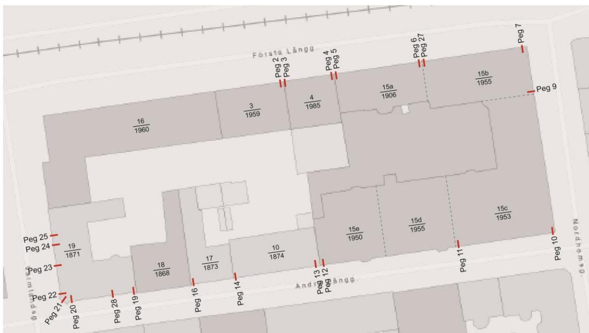
**Figure 6** Quarter Kryssaren, Masthugget, location of buildings and metal pegs.
