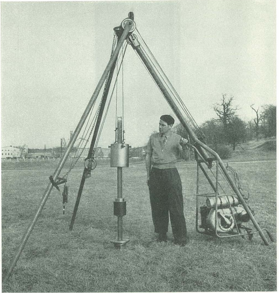
Fig. 17. Kallstenius's Sampler. Assembly for handling the sampler.
