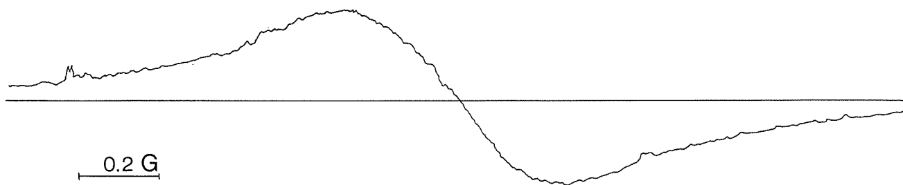
FIG. 44 Proton resonance wide line of natural Skå-Edeby clay from 2 m depth. Water content about 5 %.
