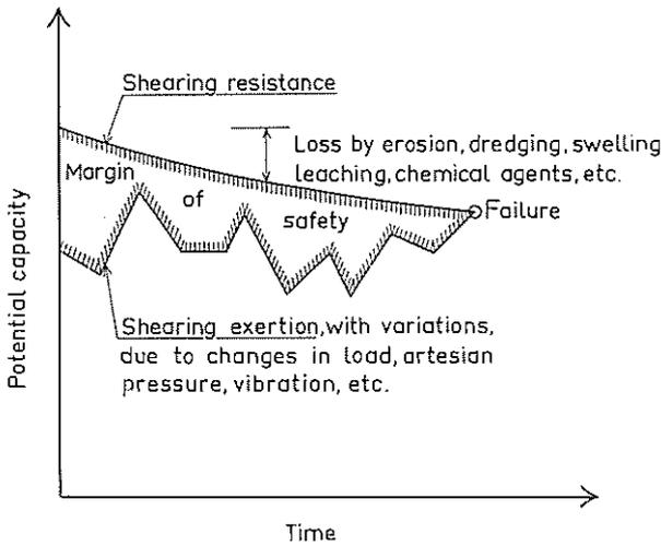
Fig. 12. Variation of shearing resistance and exertion as a function of time, in principle.
