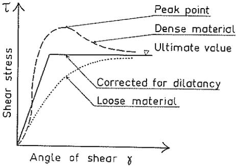
Fig. 5. Relation between stress and angle of shear obtained from shear test on friction soil.
