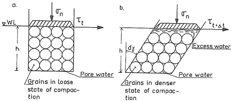
Fig. 6. Effect of undrained shear of swayable box. Container (a) with loosely filled grains and water before shear, (b) with grains in denser state after shear.
