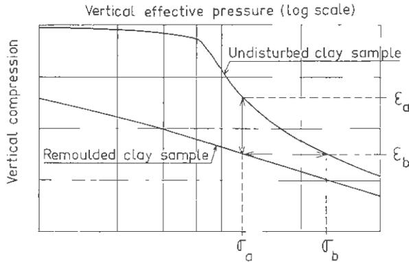
Fig. 9. Relation between results of undisturbed and remoulded clay consolidated in oedometer. The difference is shown in resistance to external load at one water content, and in internal soil structure at the same vertical effective pressure.
