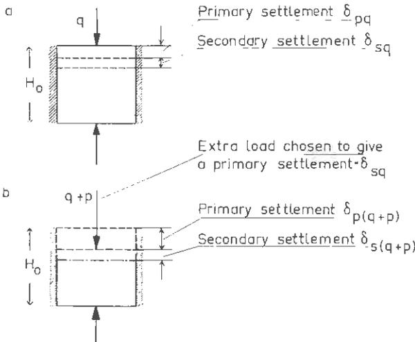
Fig. 2. Soil element, (a) subjected to primary and secondary consolidation, and (b) loaded by an additional load which, theoretically, should result in small changes of pore water pressures.
