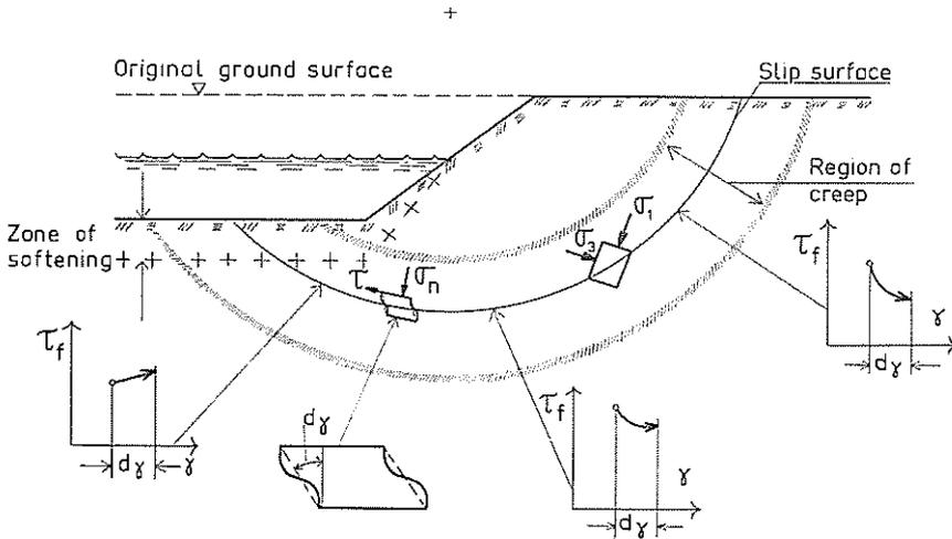
Fig. 13. Possible differences in the relationship between resistance  $\tau_f$  and average shearing  $d\gamma$  during the critical time.
