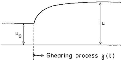
Fig. 11. Variation of pore water pressure during the shearing process, in principle.
