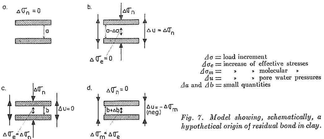
Fig. 7. Model showing, schematically, a hypothetical origin of residual bond in clay.
