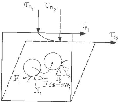
*Fig. 3. Soil element showing positions of working stresses and reactions in different stages of shearing travel at failure.*
