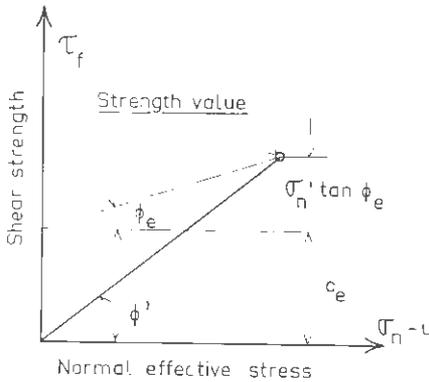
Fig. 1. Figure showing a certain strength value plotted against the effective stress in the modified Coulomb representation, and its separation, according to Hvorslev, in the effective cohesive and effective frictional components (normally consolidated clay).
