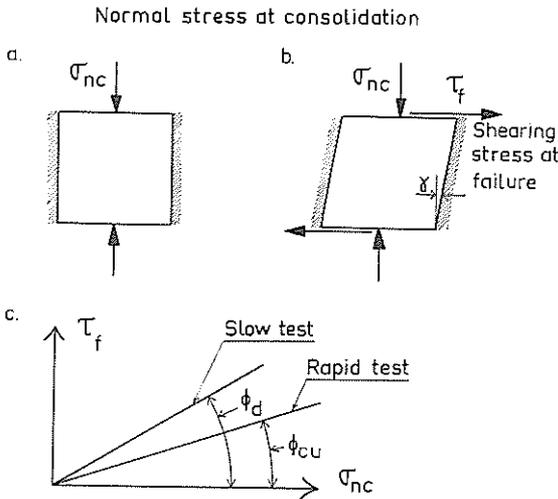
Fig. 8. Element of shear box specimen, (a) before and (b) after shearing; (c) relation between shearing resistance and normal stress at consolidation during slow and rapid tests.
