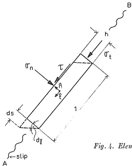
Fig. 4. Element of slip layer, AB, before and after shear.
