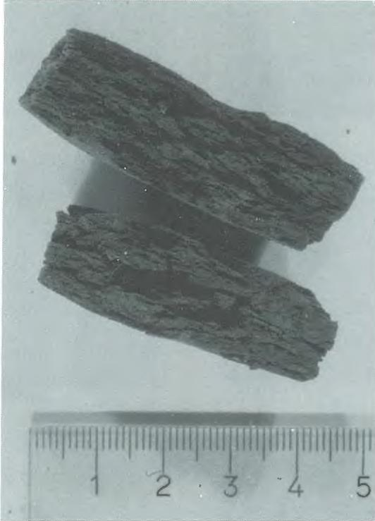
*Fig. 27. Photograph of a freeze-dried sample broken to give a vertical fracture surface. The original diameter of the sample was 50 mm.*
